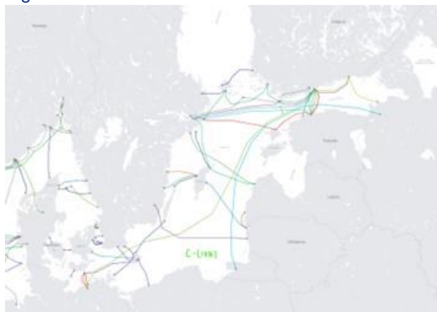
Figure 52: Finland submarine telecom cables
