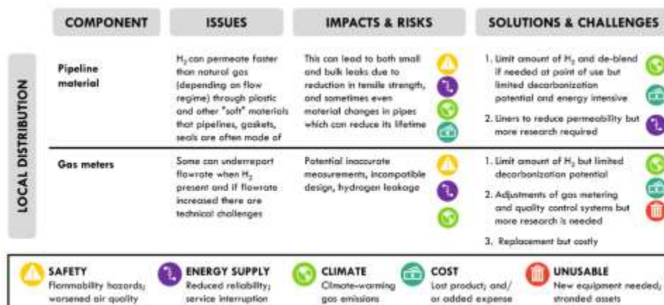
Figure 3. Local Distribution Issues With Hydrogen. Source: Energy Science and Engineering
