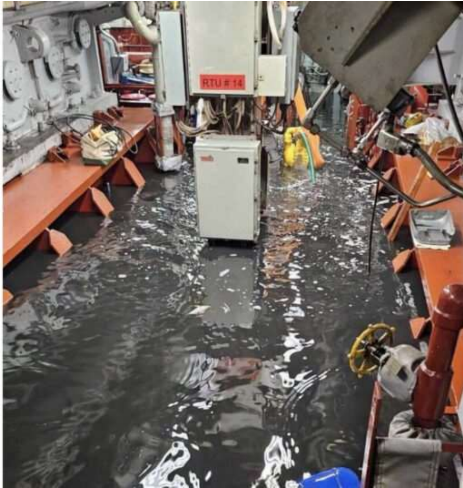
Image of a flooded mechanical space aboard the USNS Big Horn after grounding incident.
