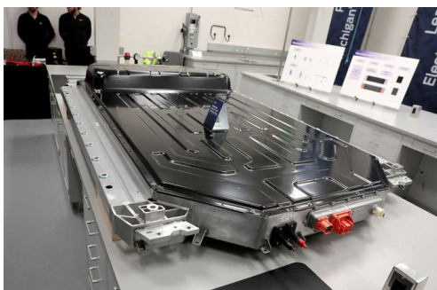
A battery pack for a Ford Mustang Mach-E. PHOTO: REBECCA
