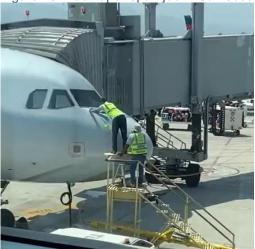
Figure 70: Duct tape repair job in San Jose del Cabo
