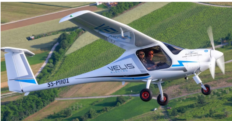
Pipistrel developed the Velis Electro, the first electric-powered airplane to receive a Type Certificate. Photo: Pipistrel.
