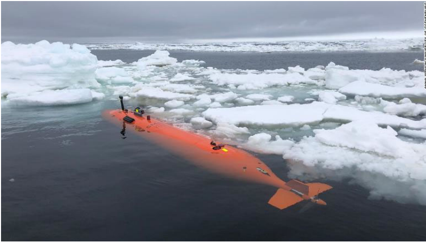
Rán, a Kongsberg HUGIN autonomous underwater vehicle, near the Thwaites Glacier after a 20-hour mission mapping the seafloor.
